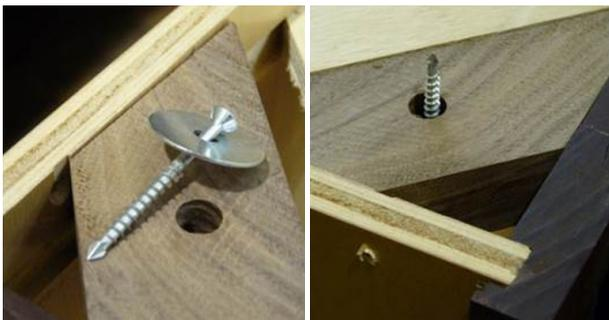
Proper screw and fender washer preparation
